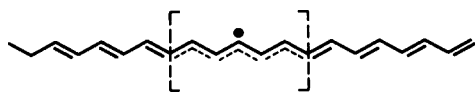
Figure 11. Soliton junction between domains in polyacetylene. The dot is an unpaired p electron. Note that the double bonds have opposite phases left and right of the junction.
